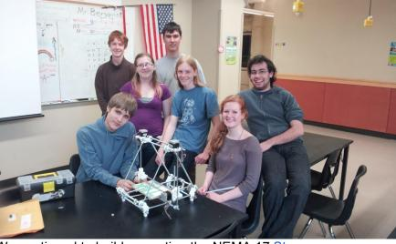
We continued to build, mounting the NEMA 17 <u>Stepper Motors</u> we bought from <u>XYZ Printers</u>. We mounted our print base after scavenging boards from GHS Tech Theatre, and used <u>pulleys and belts</u> to attach the bed to our y-axis stepper motor. Our stepper motor axles were also too small for our printed couplings, but we solved this by thickening the axles
